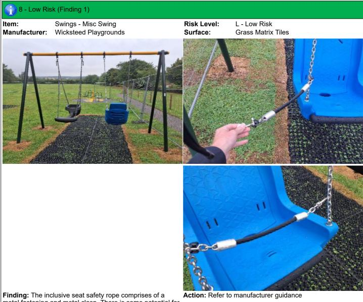
**Finding:** The inclusive seat safety rope comprises of a metal fastening and metal clasp. There is some potential for the rope to not be secured when in use and strike users
